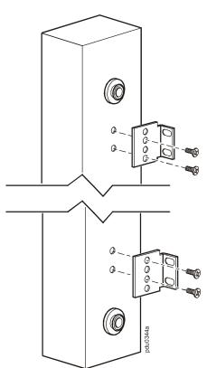
2. Install the Rack PDU on a vertical mounting rail in your rack or enclosure using the supplied screws and caged nuts with your enclosure.
