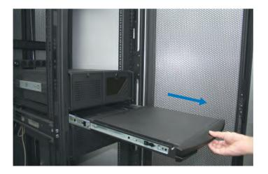
Pull the tab on the front handle and gently slide out the drawer.
