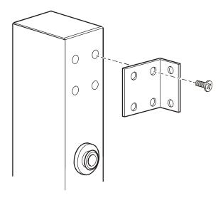
2. Install the Rack PDU on a vertical mounting rail in your rack or enclosure.
