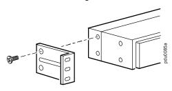
2. Install the PDU using hardware included with your rack or enclosure. The PDU will occupy one U-space.
