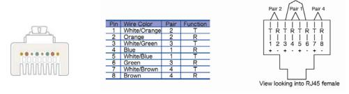
Figure 1-6. CAT5/5E/6 Straight Through UTP/STP Cable (8P8C)
