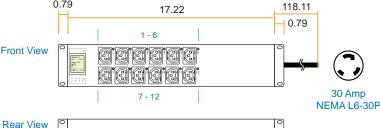
Cordset 3 meter UL 10AWG cable with 30 Amp NEMA L6-30P plug
