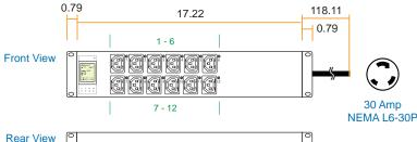
Cordset 3 meter UL 10AWG cable with 30 Amp NEMA L6-30P plug
