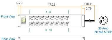
Cordset 3 meter UL 10AWG cable with 30 Amp NEMA 5-30P plug
