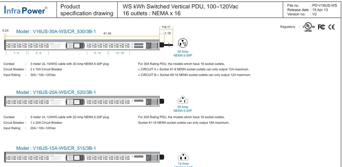
Cordset : 3 meter UL 14AWG cable with 15 Amp NEMA 5-15P plug
