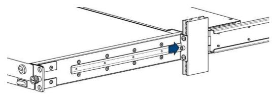
5. Install a screw to combine blocker and console. (Both sides)
