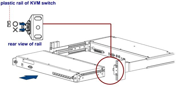
3. Tight thumb screw of bracket up to fix KVM switch in console and finish installation. (Both sides)
