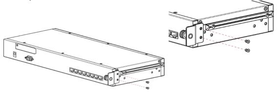
2. Push KVM switch into the rails from rear of cabinet.
