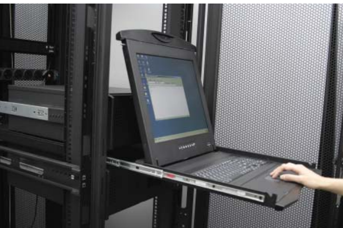
Figure 6. Operating the LCD keyboard drawer
