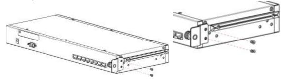
2. Push KVM switch into the rails from rear of cabinet.
