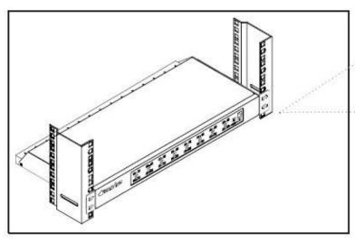
Figure 2. Fixing the KVM into the rack.
