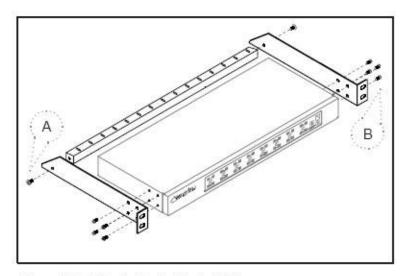
Figure 1. Installing the bracket to the KVM.
