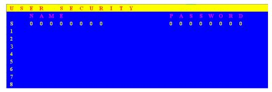
Press the **Enter** key or right button of mouse for editing. The left-top "S" means SUPERVISOR, and "1", "2", "3",..., "8" mean USERs. The maximum length of NAME and PASSWORD is eight characters (A~Z and 0~9).
