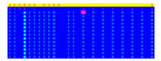
Only SUPERVISOR can configure the ACCESS LIST. The first column is the port number, following the server/computer name list. The last 8 columns are the access right of each user. Use the **Enter** key or left button of mouse to active/deactivate the access right of each port. "**X**" means to disable access and "**O**" means to enable access.
