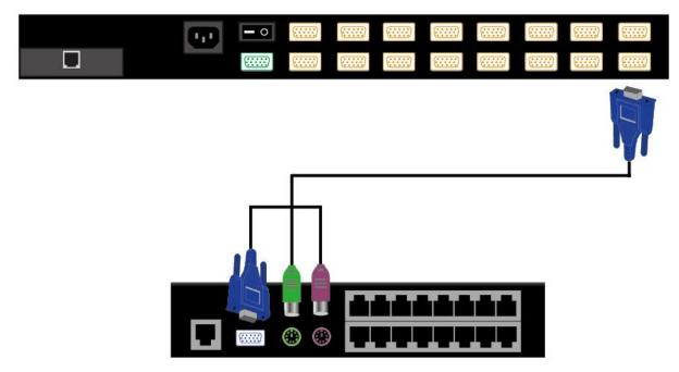
Figure 6. Cascade through Computer Port
