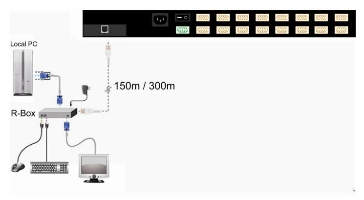
Figure 4. CAT. 5 Module Diagram
