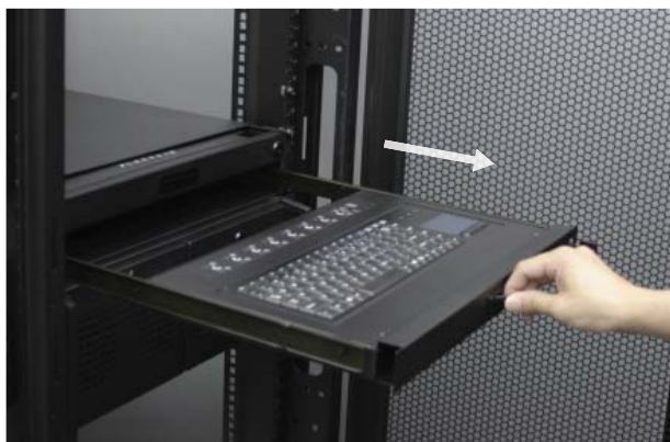
Figure 4. Pulling the handle toward the front of keyboard drawer.
