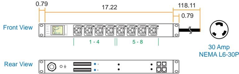
Cordset : 3 meter UL 10AWG cable with 30 Amp NEMA L6-30P plug
