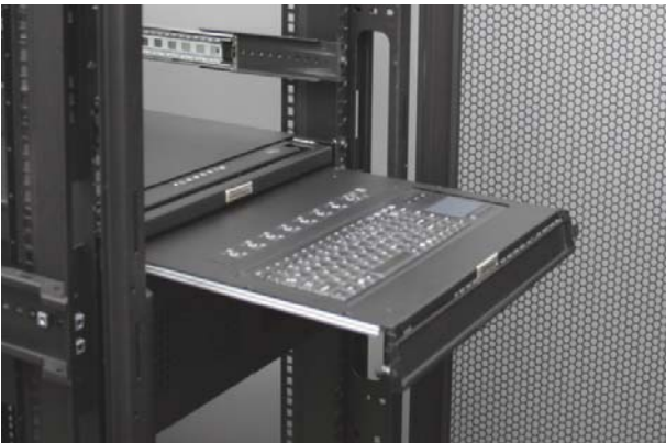
Figure 6. Pushing the upper LCD drawer until it is located in the rack.
