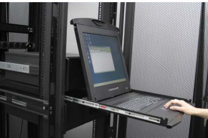
Figure 6. Operating the LCD keyboard drawer
