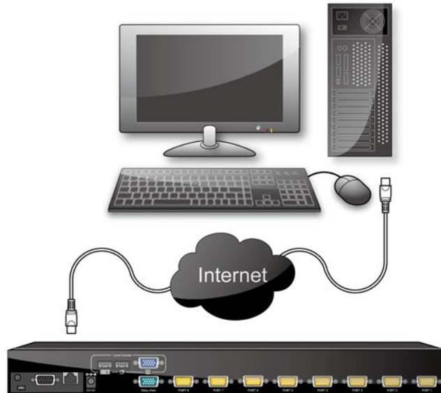
Figure 2-7. IP Module Installation
