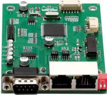
The RS-232C is used for the communication between the PC and the first display via a 15 feet serial cable while the CAN bus is used for the various LCD displays cascade together via CAT 5/6 cable, and daisy chain up to 1,000 meters.
