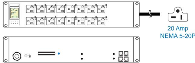
Cordset : 3 meter UL 12AWG cable with 20 Amp NEMA 5-20P plug
