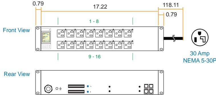
Cordset : 3 meter UL 10AWG cable with 30 Amp NEMA 5-30P plug
