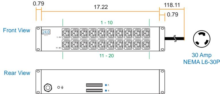
Cordset : 3 meter UL 10AWG cable with 30 Amp NEMA L6-30P plug
