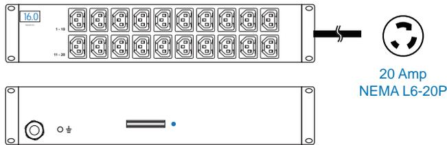
Cordset : 3 meter UL 12AWG cable with 20 Amp NEMA L6-20P plug
