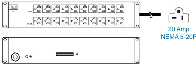
Cordset : 3 meter UL 12AWG cable with 20 Amp NEMA 5-20P plug
