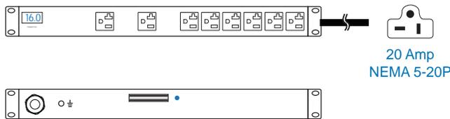
Cordset : 3 meter UL 12AWG cable with 20 Amp NEMA 5-20P plug
