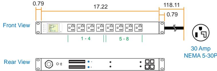
Cordset : 3 meter UL 10AWG cable with 30 Amp NEMA 5-30P plug
