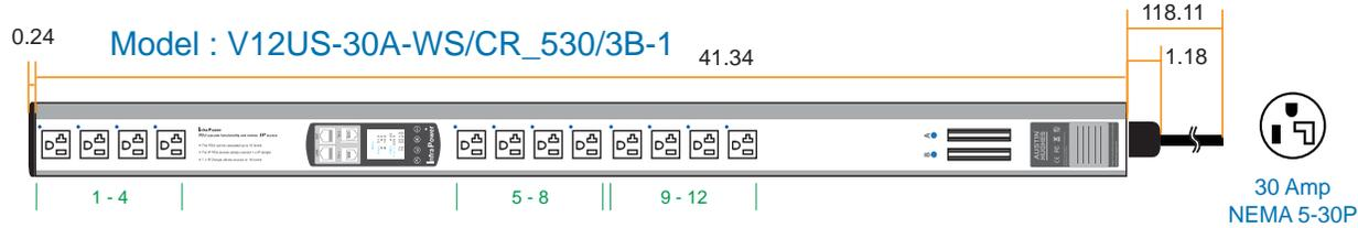
Cordset : 3 meter UL 10AWG cable with 30 Amp NEMA 5-30P plug
