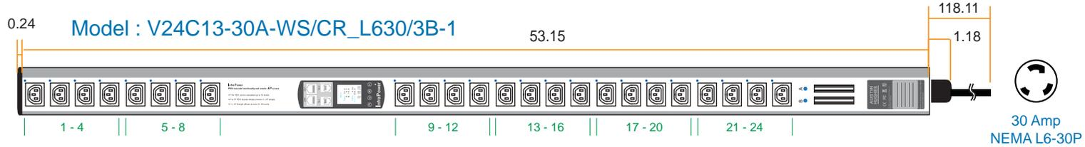
Cordset : 3 meter UL 10AWG cable with 30 Amp NEMA L6-30P plug
