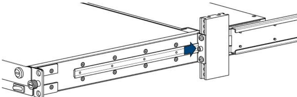
5. Install a screw to combine blocker and console. (Both sides)
