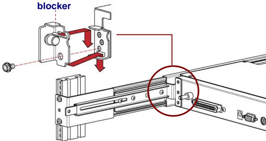
6. Install three screws (length = 6 mm) in rear of the console (Both sides) to finish the installation.
