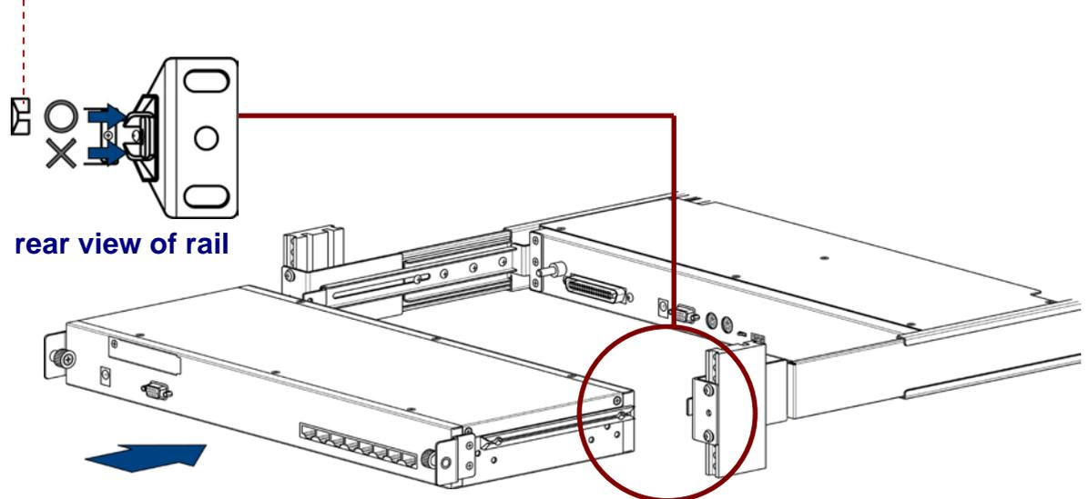
3. Tight thumb screw of bracket up to fix KVM switch in console and finish installation. (Both sides)
