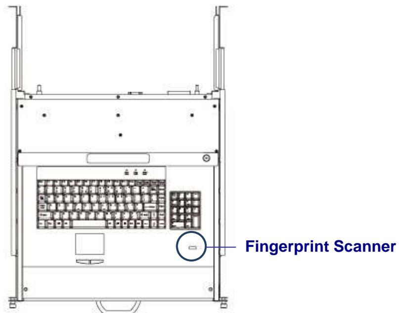
Figure 3-4. Fingerprint Scanner
