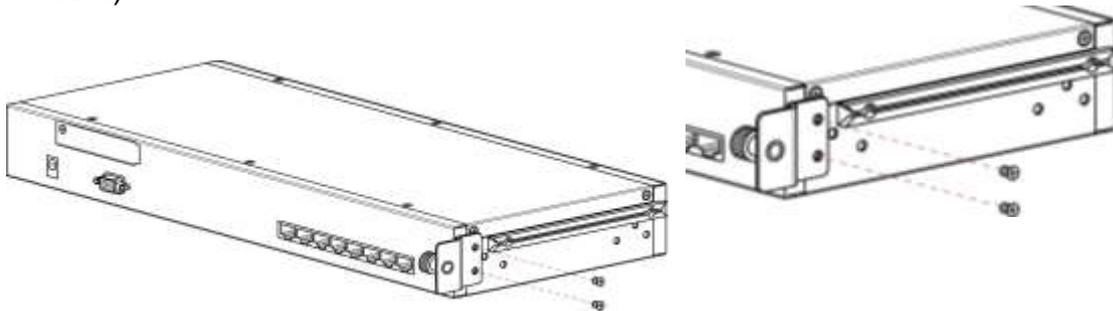
2. Push KVM switch into the rails from rear of cabinet.
