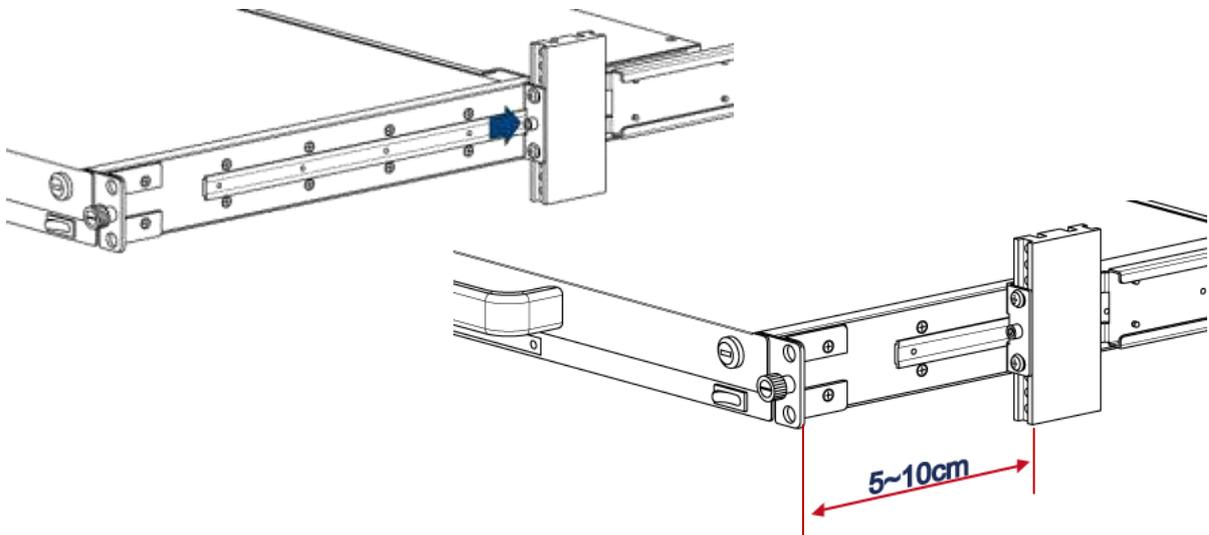
5. Install a screw to combine blocker and console. (Both sides)
