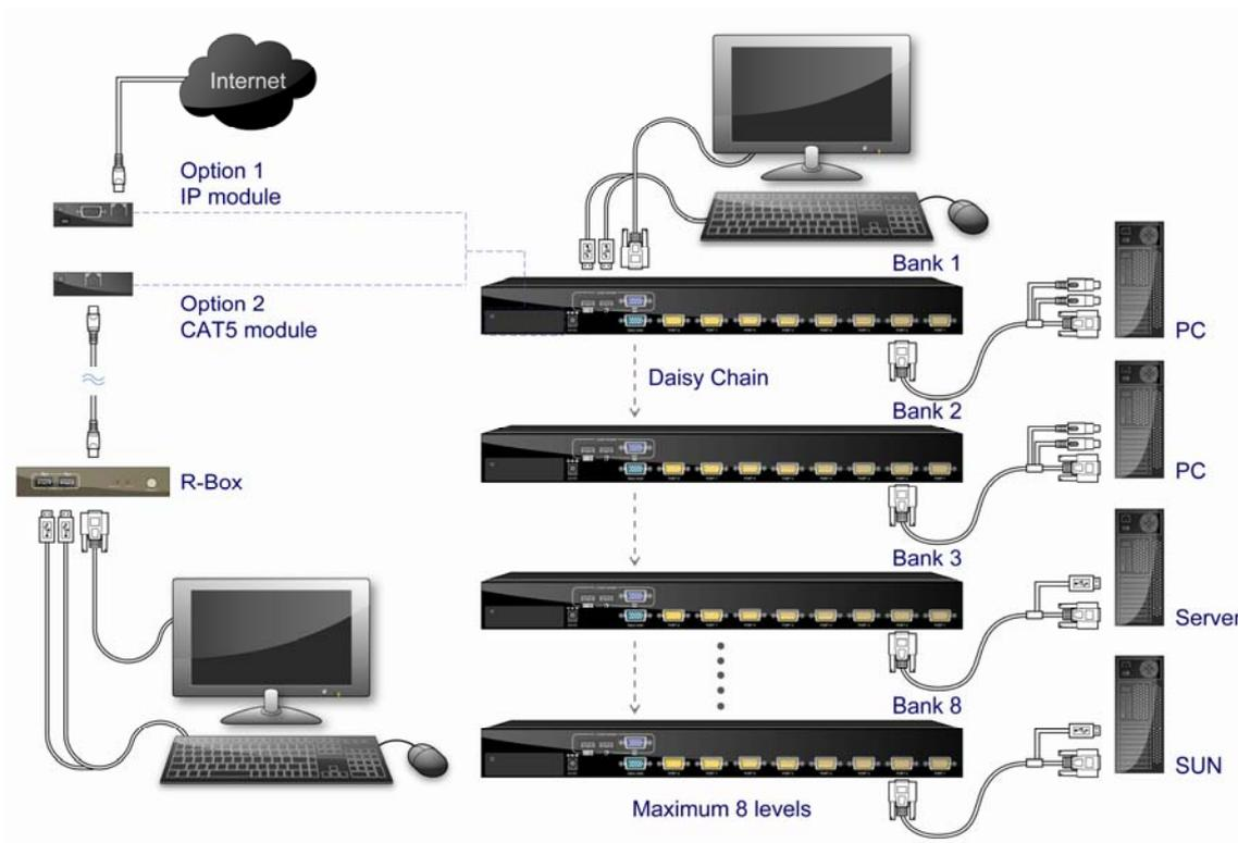
Figure 2-2. Computer / Server Installation
