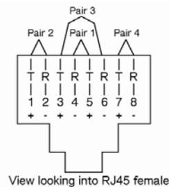
Figure 1-4. CAT5/5E/6 Straight Through UTP/STP Cable (8P8C)
