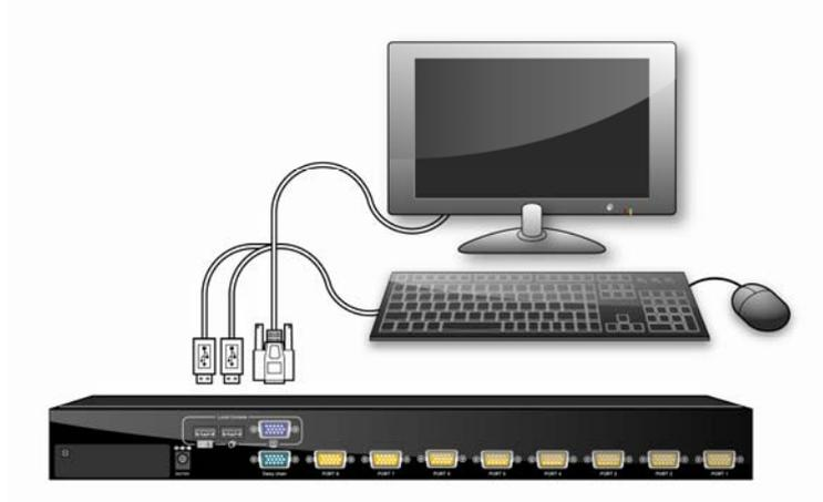
Figure 2-5. Console Installation
