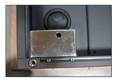
Slide the nuts to proper location.
