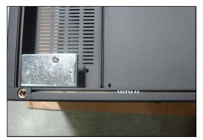
There are four screw nuts on each side of rails.
